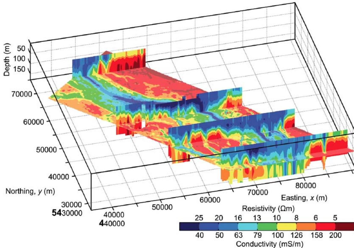
**Figure 2.** CDI model of HTEM data of Spiritwood Buried valley. The long blue-stripped feature extending NW-SE is associated with a buried valley filled with less conductive material. Red is generally bedrock. Valley fill is diamicton, clay and sand and gravel. From Oldenborger et al., (2013).
